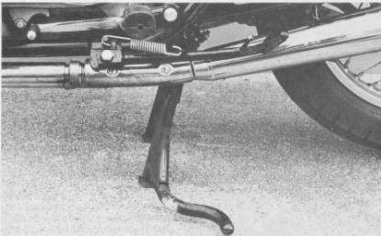
The centerstand foot bar grounds on hard left-handers, often making the rear of the bike skitter around.
