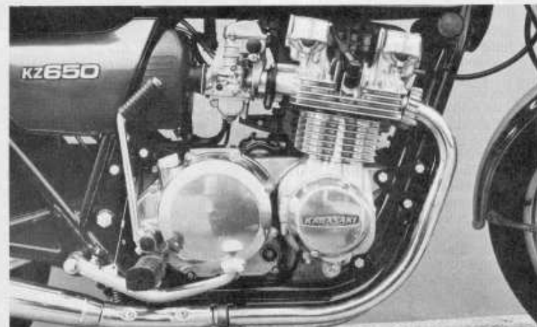
The 652cc engine is powerful for its size in the 3500 to 8500-rpm powerband, although the response is a little weak below that speed.
