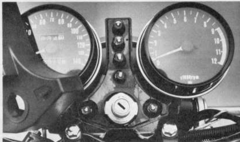
Replacing the idiot-light bulbs is simple. Just unscrew the plastic ring around the ignition switch and pop the light cover off.
