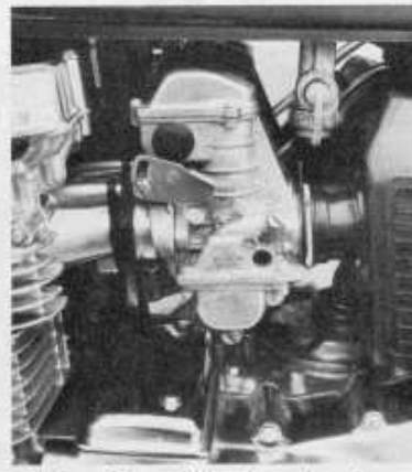
The four 24mm Mikunis carburete crisply when the engine is warm, but the KZ is extremely cold-blooded and reluctant to respond until it reaches full operating temperature.
