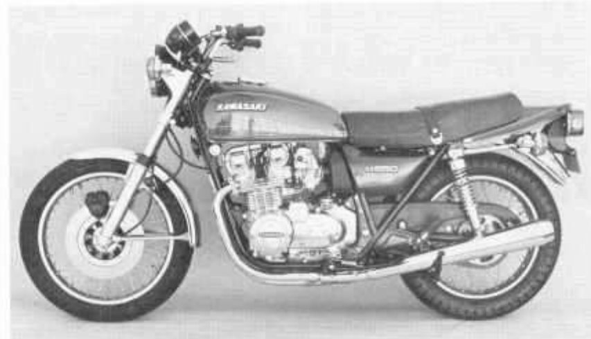
Kawasaki wanted a quiet-running engine, so the near-49-horsepower 650 features Hy-Vo chain, primary drive and a plain-bearing crankshaft. The new KZ has a space-efficient 4-into-2 muffler.
