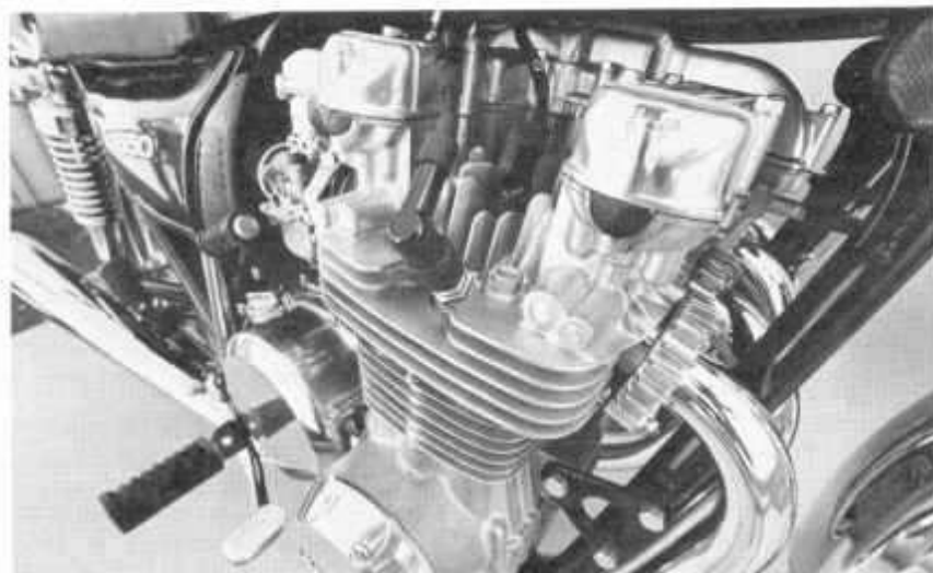
Kawasaki wanted a quiet-running engine, so the near-49-horsepower 650 features Hy-Vo chain, primary drive and a plain-bearing crankshaft. The new KZ has a space-efficient 4-into-2 muffler.
