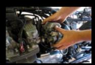
9. Removing the carbs is arguably the trickiest part of the stripdown. The still air box, which is now free of its mounting points on the battery carrier, can be shoved backwards half an inch to give a little more room, but the inlet rubbers between the carbs and filter have hardened with age and exposure to petrol vapour and lost much of their flexibility. A few minutes of determined waggling finally gets them free without damaging anything.
