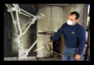
5. With the frame hooked up in the coating room Andy can now spray on the black powder. The frame is earthed and the powder particles electrostatically charged, so they adhere to the metal when they hit. However it's still a very skilled job getting into all the nooks and crannies on a bike frame and making sure everything is evenly covered.
