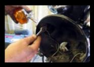
14. Up at the front end the headlamp shell is retained by the winker stems, which pass through rubber grommets in the headlamp brackets and each have single nuts at the back. With the winkers removed the shell lifts clear.
