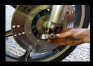
22. At the sharp end the front wheel is retained in the fork legs with two alloy clamps, again there's no need to remove the wheel spindle at this stage. These clamps can sometimes corrode in place, but these have been copper slipped fairly recently.
