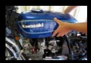
3. The Z650 tank is simply push fitted into a rubber grommet on the frame, so I can now pull it up and backwards to release it from the two rubber bobbins at the headstock. The tank gets wrapped up and stored for safety for the time being.
