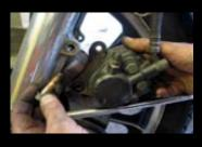
17. Mark wants a twin disc set up fitting when the bike is rebuilt. I'll probably be re-building and re-using this left hand caliper, which looks in reasonably good nick. Signs of copper slip on the mounting bolts are very encouraging, but I reserve final judgement until I try to free off the bleed nipple.
